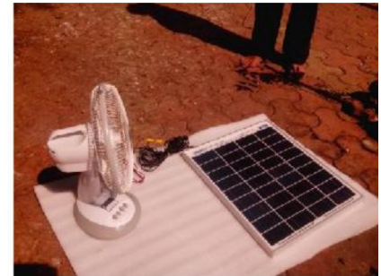
Connect the wire of Solar Panel and Solar Fan.
